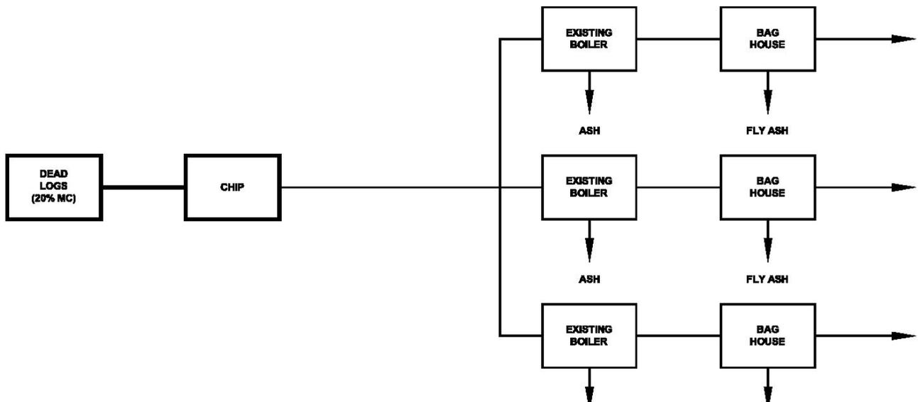
The third option for burning biomass (Generation Option No. 5) includes the use of green (wet) logs with a moisture content of
