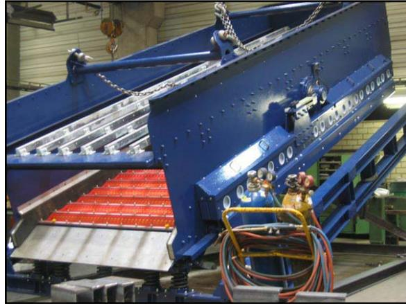
The use of separator screens will provide two streams of coal feed. The existing boilers will be fed stoker grade coal per their original design. The coal fines will be separated and can be re-processed back to the mine, sold to a third party such as Mountain Cement, or fed to an auxiliary pulverized coal burner or boiler as illustrated below:
