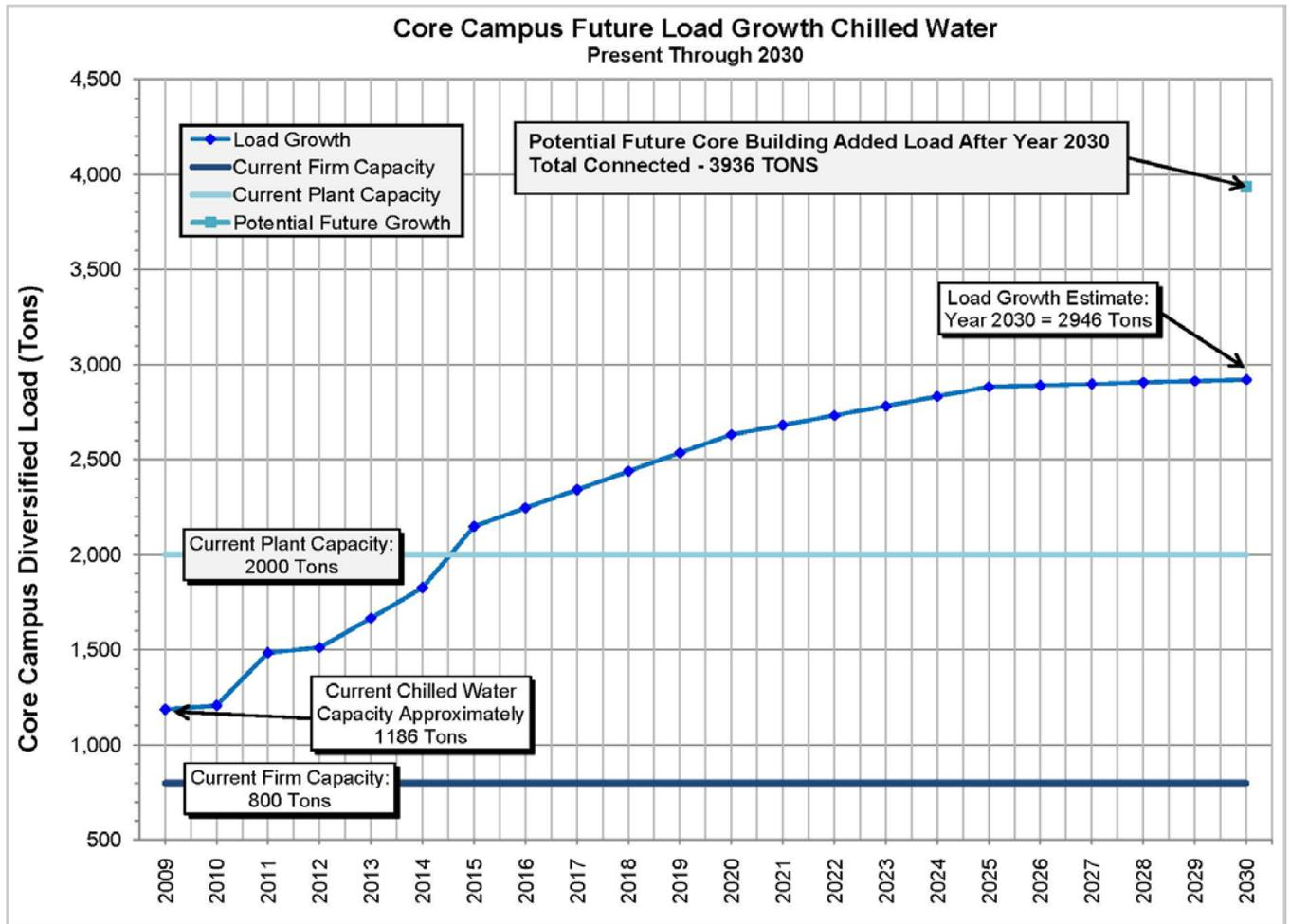
Utility distribution has been evaluated in Section III and is adequate to sustain additional load up to 2500 tons within the 14" pipe immediately from the CEP. This capacity is based on a 14° delta and maximum pipe velocity of 10fps. Additional information can be found in Table IV-D-1 for evaluation of future loads through pipes in comparison to delta T of the chilled water system.
